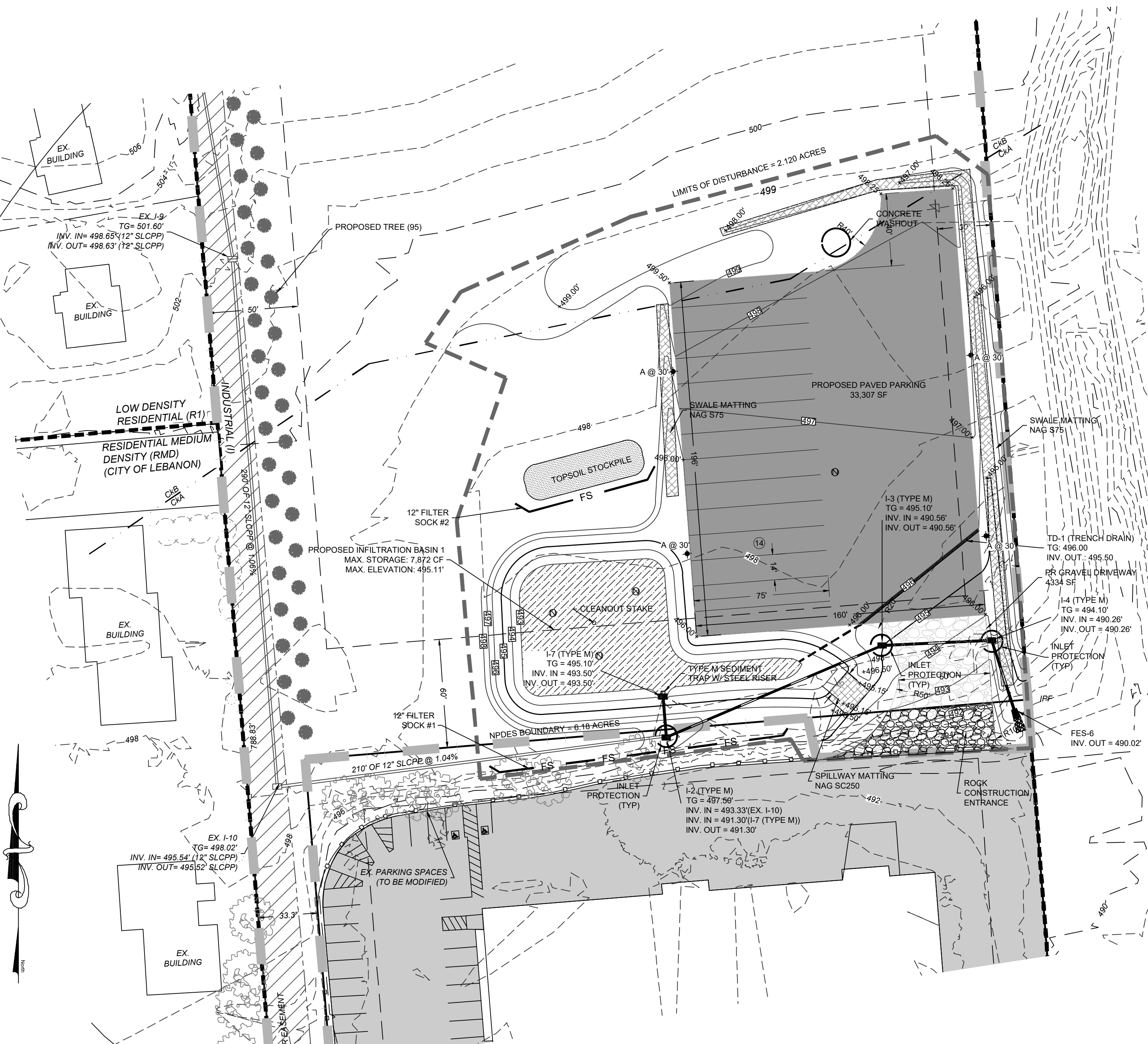
EROSION & SEDIMENT POLLUTION CONTROL PLAN 1"=40'
