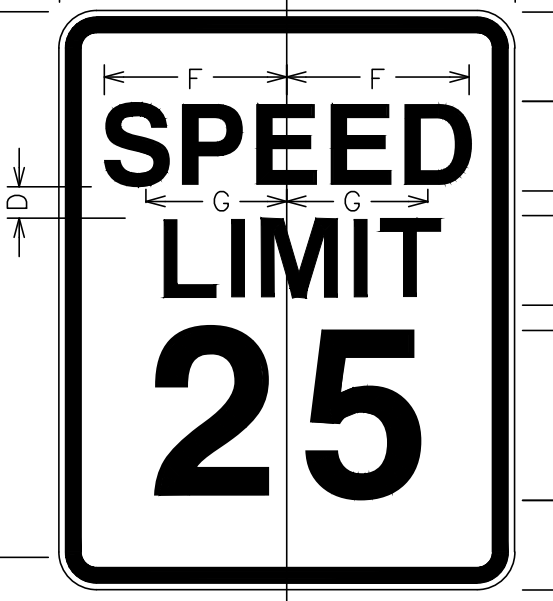
SPEED LIMIT SIGN DETAIL
